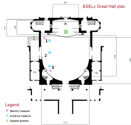
Figure 7 - ESELx Great Hall – measurement points and source location.
