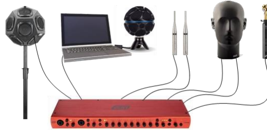
Figure 1 - RIR acquisition hardware
